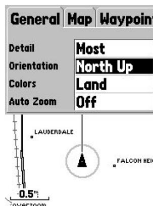
20. Highlight the 'Orientation' field and press <ENTER> to view the options. Select 'Course Up' using the <ROCKER> key, press <ENTER> to accept your changes, and press the <PAGE> key to return to the 'Map View' screen.
