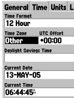
8. *Ensure you reset the time zone back to Central by highlighting the 'Time Zone' field, pressing the <ENTER> key to display the time zone options, using the <ROCKER> key to highlight 'Central' and pressing the <ENTER> key.*
