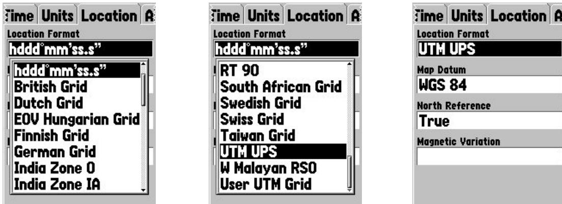
7. Press the <PAGE> key to accept the changes and return to the 'Satellite' screen where you will see the UTM coordinates for the current position fix.
