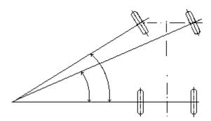
This allows both tires to roll around a common point in a corner or curve and greatly improves cornering ability, performance and reduces tire wear. Rudolf Ackerman patented his design of angled steering arms in England in 1818 for horse drawn carriages. Before this principle was developed horse drawn carriages were fitted with parallel steering arms and suffered from poor steering performance. Since then Ackerman Steering has had a huge impact on many different vehicles.
