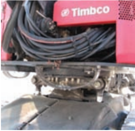
This is an example of additional steps added to mobile equipment for maintenance purposes.
