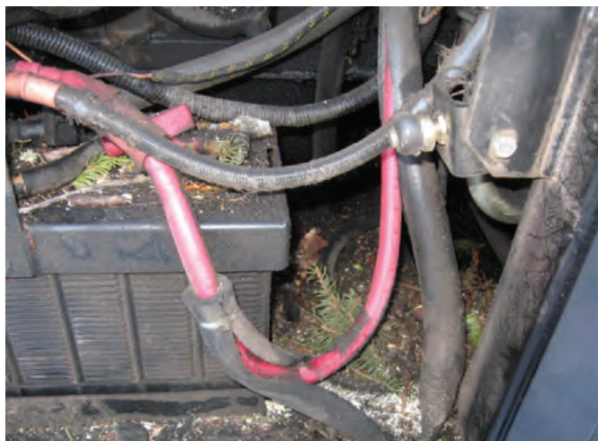
This picture shows where daily housekeeping would improve fire and personnel safety as well as being able to uncover maintenance needs.
