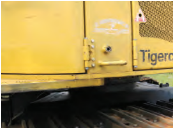
Example of discharging outside the engine and hydraulic compartments – recommended.
